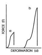
Fig. 2. Typical compression curves of mealy grain (a) and vitreous grain (b).
